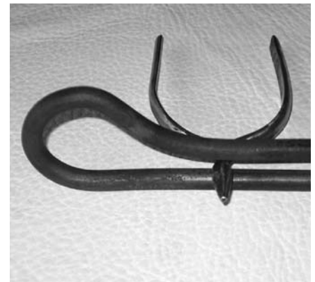
FIGURE 8 photo by David Cadwell | Agelos Eviennece Necking down the metal using a fuller tool.
