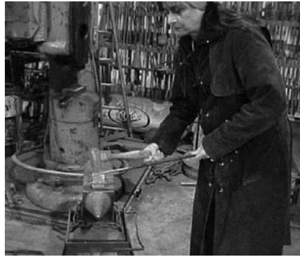
FIGURE 5 photo by David Cadwell | Agelos Eviennece Using a bronze hammer to pound open the split in the hammer.
