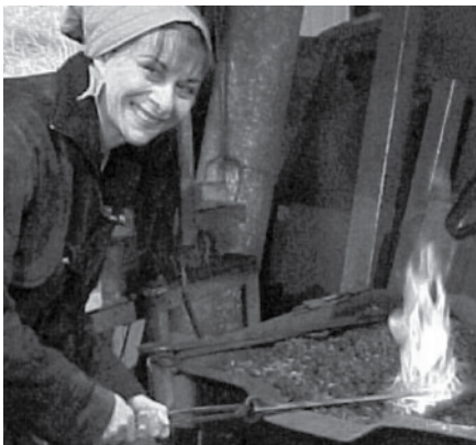
FIGURE 2 photo by David Cadwell | Agelos Evienece Author heating bar stock at the forge.
