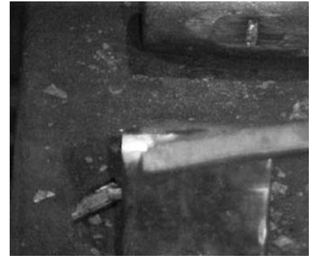
FIGURE 6 photo by David Cadwell | Agelos Eviennece The heated metal is worked on top of a stationary chisel.
